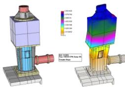
**Operational Deflection Shape Analysis** - Time or frequency based Operational Deflection Shape (**ODS**) is used to analyze the motion of rotating equipment and structures. An ODS animates a computer-generated model of the machine with phase and magnitude data or simultaneously measured time waveform captures. ODS is a non-intrusive testing technique.
