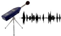
**Sound/Noise** – Airborne noise measurement used to diagnose vibration on rotating machines or to investigate neighborhood noise complaints, or document fence-line noise and human exposure levels.
