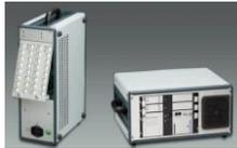
**Short or Long-Term Monitoring** – Short or long-term monitoring of vibration or process signals. Monitoring instrumentation is 24 channels and is capable of measuring and storing long time waveform captures, trends, spectrums, waveforms.
