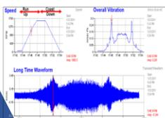
**Resonance Testing** – Resonant amplification (Resonance) results whenever forced vibration, from mechanical faults, coincides with a natural frequency. A natural frequency is the frequency or frequencies that a machine “likes” to vibrate or “ring”. At resonance, a small change in the exciting force produces a large change in vibration.
